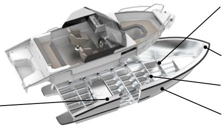
Reinforcing beams and strengthening cross sections in the hull, gives the boat exceptional torsional stiffness.
