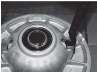
Insert hooked end of tool.
