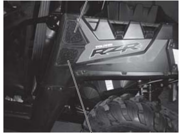
PVT Intake Pre-Filter
