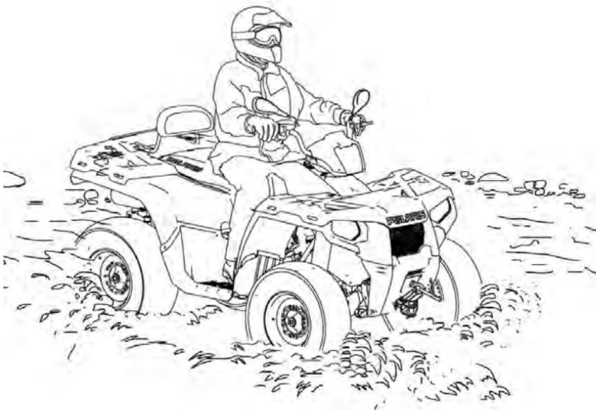
Your ATV can operate through water with a maximum recommended depth equal to the bottom of the footrests. Follow these procedures when operating through water:
