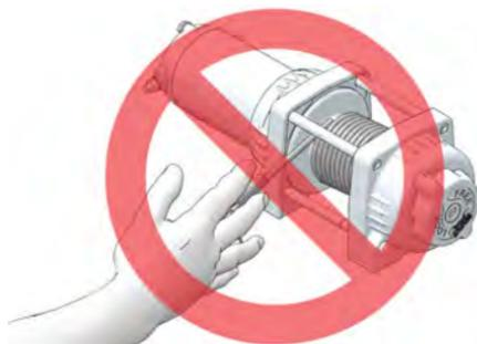
18. Never release the clutch on the winch when the winch cable is under load.
