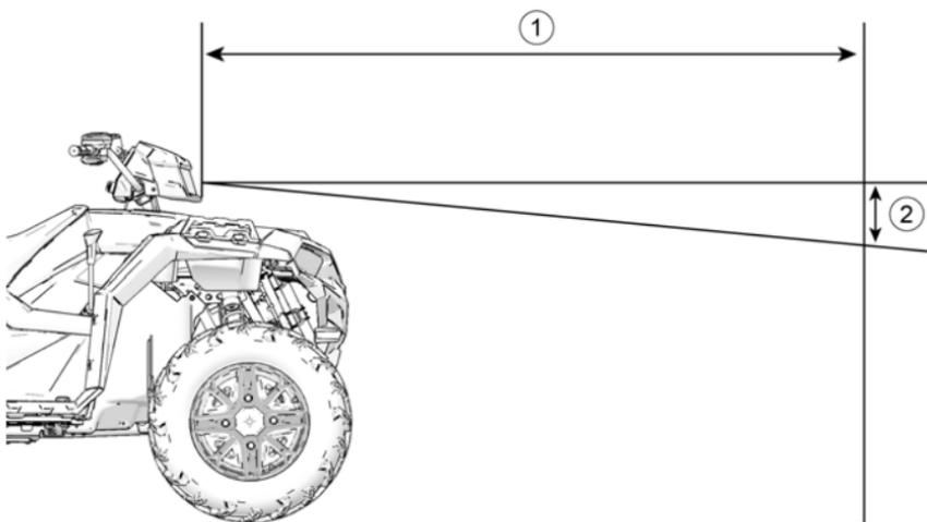
1. Position the vehicle on a level surface with the headlight approximately 25 ft. (7.6 m) from a wall ①. Place the transmission in PARK.
