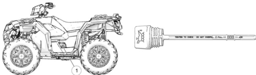
Check the oil level when the engine is cold. Never check the oil with the engine running.
