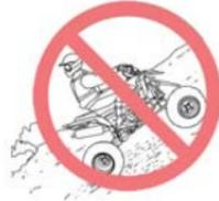
Keep weight uphill. Never apply engine power. Never apply the rear brake while rolling backwards. Apply the front brake slowly. When fully stopped, apply rear brake as well, and then lock the parking brake. Dismount on uphill side, or to either side if pointed straight uphill. Turn the ATV around and remount, following the procedure described in the Owner's Manual. See page 86.
