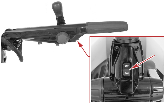
Tilt switch on tiller handle models
