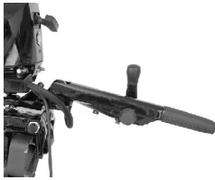
b. Adjustment knob at the highest setting.
